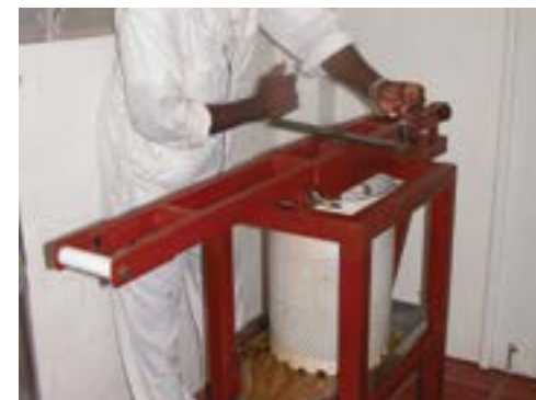
The press works by turning a large handle to increase the pressure on the honeycombs.
